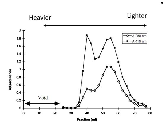
**Gel-filtration of the protein** mixture. 1.2 ml of protein mixture (10 mg/ml) was loaded onto a 25 cm X 2.5 cm diam. Sephadex G-50 column equilibrated with buffer (50 mM Tris HCl, pH 7.5). The column was eluted with buffer at ~1 ml/min, collecting 2.5 ml fractions. The absorbance of each fraction was measured at 280 nm.
